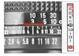
There are two ways to check depth of field. One is by using the depth-of-field scale on the lens. This is a scale of f/stops repeated on each side of the distance index.
