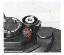
When you have reached the end of the film, the film advance lever will stop before the end of its stroke.
