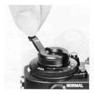
The F-1's provision for multiple exposures allows you to easily make two or more exposures on the same frame for creative effect.
