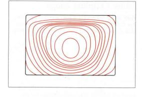
With the Canon F-1, a special optical element in each focusing screen determines the metering sensitivity area. Thus the metering area can be changed, according to the subject you are shooting and the lens in use, simply by replacing the focusing screen.
