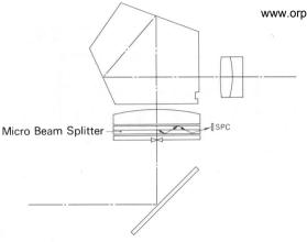
Since the optical element is located in close proximity to the focal plane, this new system of metering sensitivity distribution ensures extremely accurate results.
